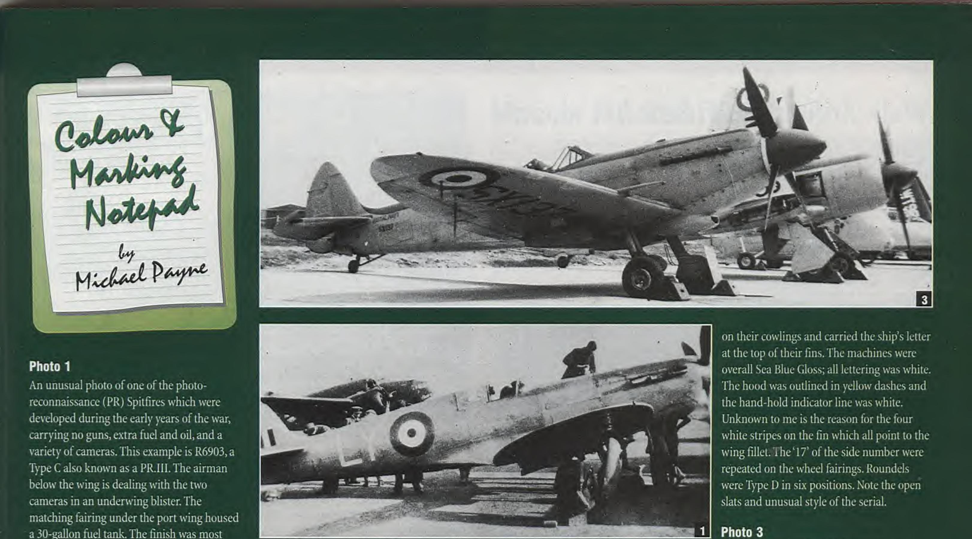
a 30-gallon fuel tank. The finish was most probably 'Camotint Pink', an elusive tone, slightly mauve, but effective for concealment at most altitudes. Note the deep forward 'chin' where there was an enlarged oil tank, the clear, rounded windscreen and the blisters on the hood for added pilot visibility.
